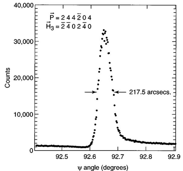
FIG. 2. Azimuthal plot of the  $(2\ 4\ 4\ \bar{2}\ 0\ 4)$  reflection, a three-beam case. The simultaneous reflection  $\mathbf{H}$  is the  $(\bar{2}\ 4\ 0\ 2\ 4\ 0)$ . The x-ray energy is 7000 eV. The azimuthal angle is zero when the  $(0\ 0\ 0\ \bar{1}\ 0)$  axis is in the scattering plane, mostly antiparallel to the incident beam, and the diffractometer angle  $\psi_0 = 249.771^\circ$ . The counting time on each point was about 1 s. The increment on  $\psi$  was  $0.002^\circ$ .
