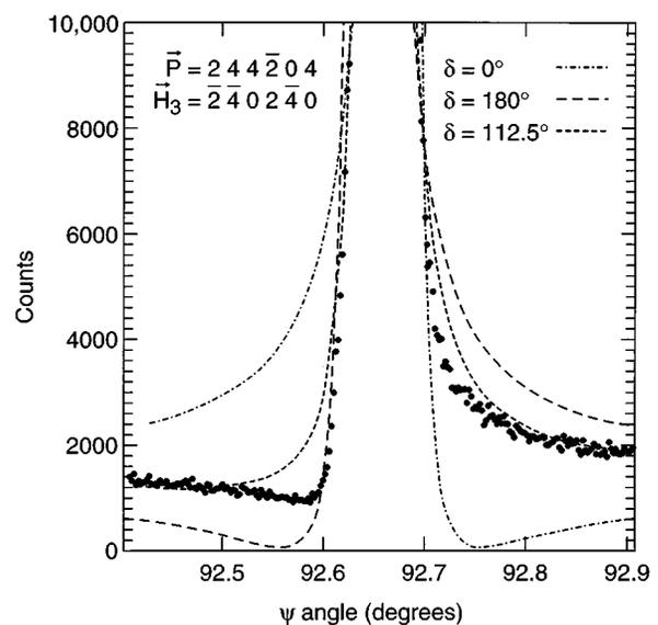
FIG. 3. The same as Fig. 2, except that the multiple diffraction peak (heavy dots) was truncated at the counting number of 10 000. The short-dashed line is a fit with a triplet invariant  $\delta = 0^\circ$ , and the long-dashed line is the one with  $\delta = 180^\circ$ . The small dashed line is the best fit, with  $\delta = 112.5^\circ$ .
