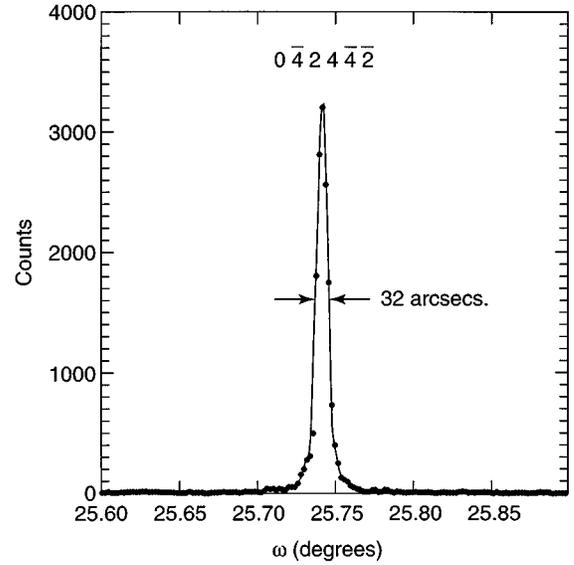
FIG. 1. Rocking curve of the  $(0\ \bar{4}\ 2\ 4\ \bar{4}\ \bar{2})$ . The counting time on each point was about 2 s. The increment  $\Delta\theta$  was  $0.002^\circ$ . The width of the rocking curve corresponds to the instrumental resolution.
